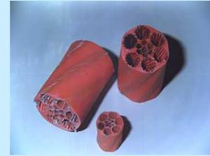
Plastic impregnated ropes have been successfully used on coal and ore unloaders and also in piling operations.
