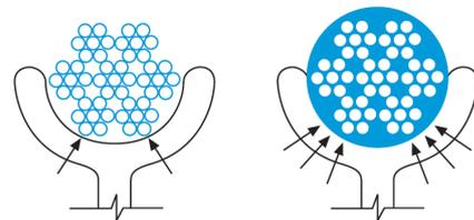
Contact of conventional wire rope with the winding drum and sheaves inevitably leads to high pressure point contact where individual wires meet the contour of the groove. With PIR rope the load is spread and wear on both the rope and drum is minimised.
